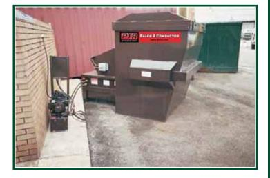
The PSC is compatible with a majority of front and rear load vehicles. The low profile makes it easier and safer for drivers to see over the unit. It features a remote power unit and a Tri-Voltage motor with quick disconnect which allows for ease of service. These features make the PCS one of the most economical and simplest to use self-contained front or rear loading containers on the market.
